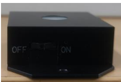
e) Probe 전원 Off 일 때 Blue Led Off Blue Led Off when Probe is powered Off
