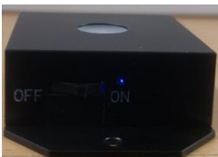
f) Probe 전원 On 일 때 Blue Led On Blue Led On when Probe is powered On
