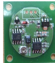
Microcurrent amplification -> Output : voltage(0~5V) or current (4-20mA)
