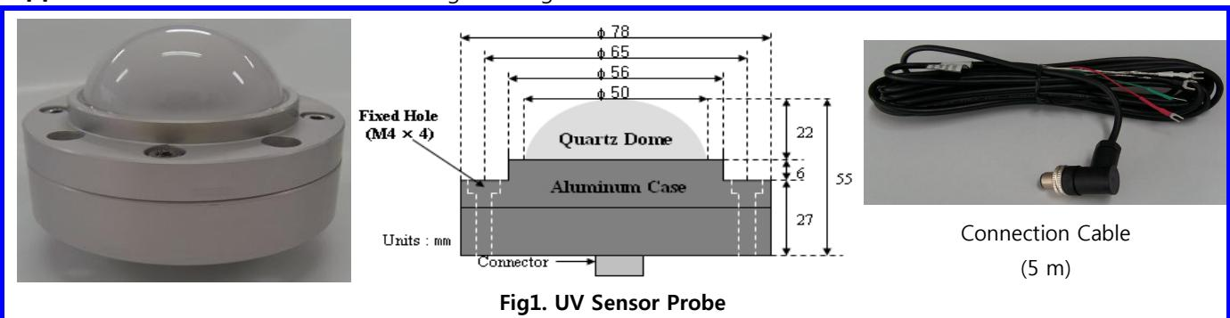
Fig1. UV Sensor Probe
